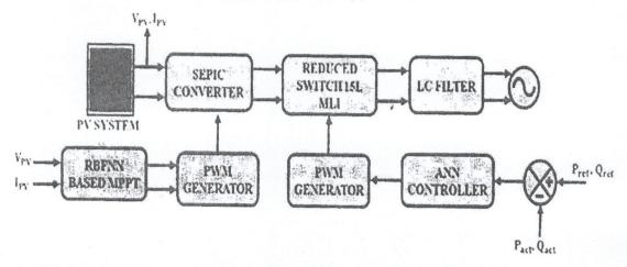
The PV system used for power adaptation is made up of numerous systems and similar arrangements of PV modules, a subsequent controller, and power converters like a DC-DC converter and inverter. As a result, the DC voltage produced may be improved using a DC to DC converter and converted to AC using an inverter. The Photovoltaic panel should be certain originated on the weight rating.
