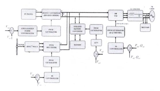
This project provides a reliable operating approach for a solar and wind hybrid power systembased MG system. Three primary components can be identified: the battery storage systems, PV and wind systems interconnected to the DC-link. The bi directional converter is incorporated to provide optimal load management using a dynamical modelling and control system powered by a PV system and wind. Using bidirectional converters, the DC bus is linked to the battery.
